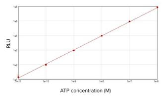
An ATP standard curve spanning five decades was run using the ATPlite 1step Luminescence Assay System (PerkinElmer) on the SpectraMax iD5 reader. Standard concentrations ranged from 1x10-11 M to 1x10-6 M. A wide linear dynamic range ensures accurate assay results across a broad span of sample types. Standards were plotted using a log-log curve fit in SoftMax Pro Software.
