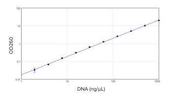
The SpectraMax iD5 reader is fully compatible with the SpectraDrop Micro-Volume Microplate, enabling quantitation of precious low-volume samples. 4- $\mu$ L DNA standards from 2 ng/ $\mu$ L to 1000 ng/ $\mu$ L were read in absorbance detection mode with a preconfigured protocol in SoftMax Pro Software. Performance matching the 2 ng/ $\mu$ L sensitivity specification is demonstrated here.
