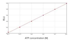
An ATP standard curve spanning five decades was run using the ATPlite 1step Luminescence Assay System (PerkinElmer) on the SpectraMax iD3 reader. Standard concentrations ranged from 1x10<sup>-11</sup> M to 1x10<sup>-6</sup> M. A wide linear dynamic range ensures accurate assay results across a broad span of sample types. Standards were plotted using a loglog curve fit in SoftMax Pro Software.
