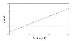
The SpectraMax iD3 reader is fully compatible with the SpectraDrop Micro-Volume Microplate, enabling quantitation of precious low-volume samples. 4- $\mu$ L DNA standards from 2 ng/ $\mu$ L to 1000 ng/ $\mu$ L were read in absorbance detection mode with a preconfigured protocol in SoftMax Pro Software. Performance matching the 2 ng/ $\mu$ L sensitivity specification is demonstrated here.
